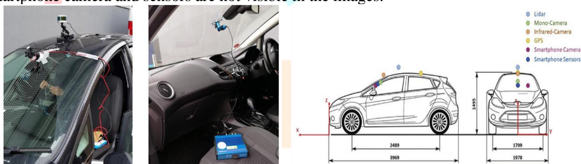
Figure 2a / 2b /2c Research vehicle exterior / interior setup / vehicle dimensions and sensor positions
