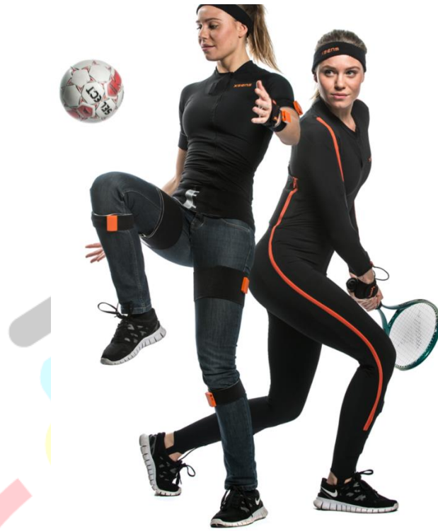
Figure 1: Xsens MVN Consisting of 17 Inertial and Magnetic Motion Trackers (Schepers, M. et al., (2018, March 23)
