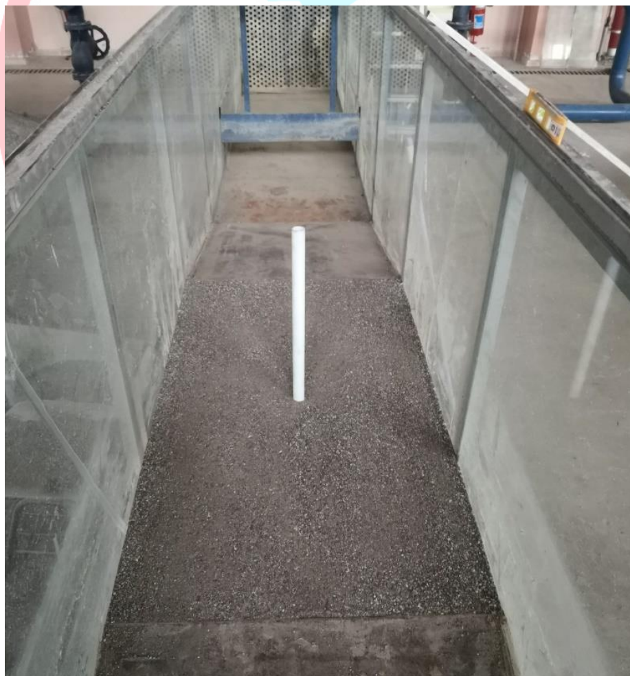
Fig. 2 Test section and Pier installation.
