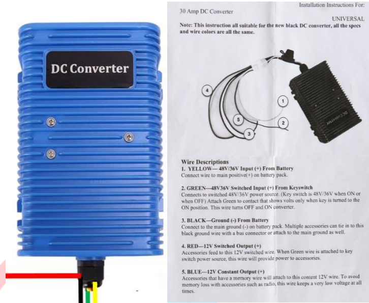
Figure 43 DC Converter Connections
