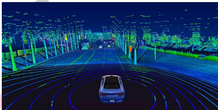
Figure 1 Three-dimensional visualization of point cloud data obtained by LIDAR (Akarsu)
